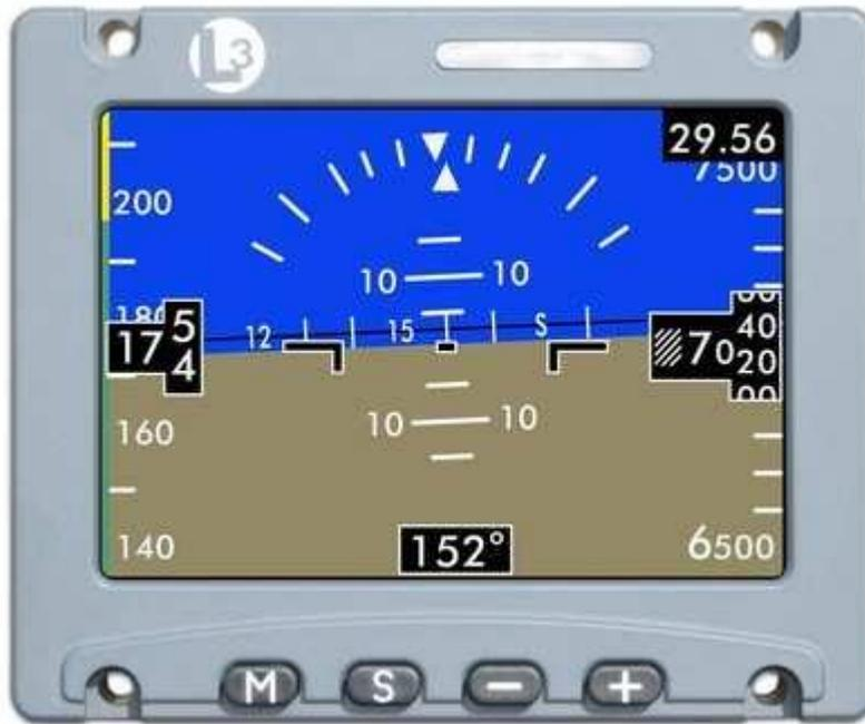
**Fig 2.13 Solid state integrated standby instruments**
