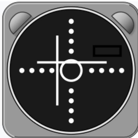
Fig 4.31: The pilot has to correct to the left and a little upwards.
